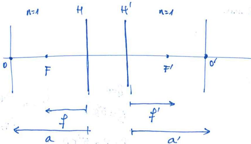
$$M_{OO'} = \begin{pmatrix} 1 & -a' \\ 0 & 1 \end{pmatrix} \begin{pmatrix} 1 & 0 \\ 1/f & 1 \end{pmatrix} \begin{pmatrix} 1 & a \\ 0 & 1 \end{pmatrix} = \begin{pmatrix} 1 - \frac{a'}{f} & (a-a') \left(1 + \frac{a}{f'}\right) \\ 1/f & 1 + \frac{a}{f'} \end{pmatrix}$$
