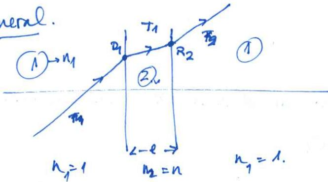
o  $M_{12} = \begin{pmatrix} 1 & 0 \\ 0 & n/1 \end{pmatrix} \begin{pmatrix} 1 & -e \\ 0 & 1 \end{pmatrix} \begin{pmatrix} 1 & 0 \\ 0 & 1/n \end{pmatrix} = \begin{pmatrix} 1 & -\frac{e}{n} \\ 0 & 1 \end{pmatrix}$
