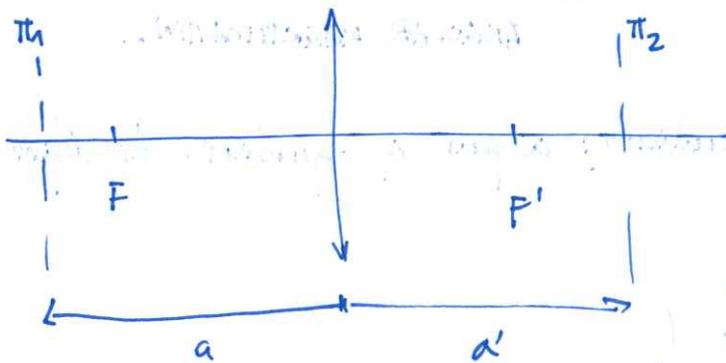
$$M_{12} = \begin{pmatrix} 1 & -a' \\ 0 & 1 \end{pmatrix} \begin{pmatrix} 1 & 0 \\ 1/f & 1 \end{pmatrix} \begin{pmatrix} 1 & +a \\ 0 & 1 \end{pmatrix} = \begin{pmatrix} 1 - \frac{a'}{f} & +a - a' - \frac{aa'}{f} \\ 1/f & 1 + \frac{a}{f} \end{pmatrix}$$
