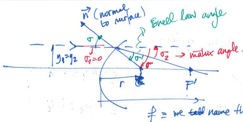
$$\sigma_2 = (\sigma' - \sigma) = \sigma \left( \frac{n_1}{n_2} - 1 \right) \stackrel{\substack{\uparrow \\ n_1 \sigma = n_2 \sigma'}}{=} \frac{y_1}{r} \left( 1 - \frac{n_1}{n_2} \right) = \frac{y_1}{r} \left( \frac{n_2 - n_1}{n_2} \right)$$
