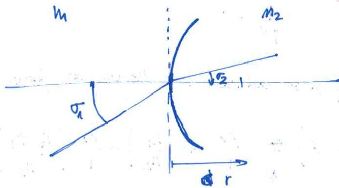
$$\left. \begin{aligned} y_2 &= Ay_1 + B\sigma_1 \\ \sigma_2 &= Cy_1 + D\sigma_1 \end{aligned} \right\}$$
