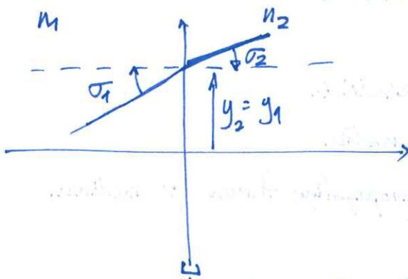
$$n_i = \frac{c}{v_i} \equiv \text{Refractive index.}$$
