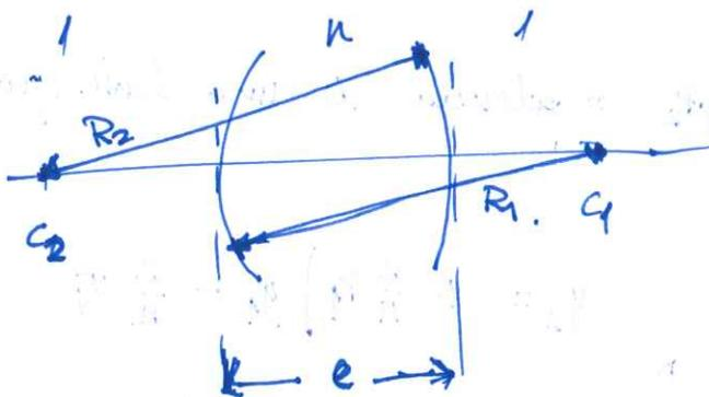
$$TL = \begin{pmatrix} 1 & 0 \\ 1/R_2 & n \end{pmatrix} \begin{pmatrix} 1 & -e \\ 0 & 1 \end{pmatrix} \begin{pmatrix} 1 & 0 \\ 1/f_1 & 1/n \end{pmatrix}$$
