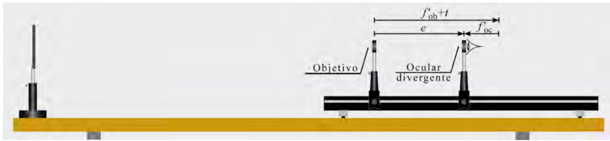
Figure 4.5 Diagram of a Galileo's telescope.
